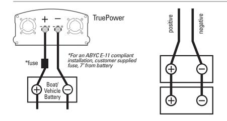
**Figure 1)** This wiring setup displays an inverter connected directly to the engine battery for light-duty applications. **Figure 2)** Displays 2 x 12volt batteries connected in a parallel system that doubles the capacity and maintains the 12v voltage requirement of your inverter. This battery bank requires a battery charging system.
